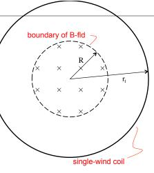
What we know from Faraday's Law: When the magnetic field changes through the face of the coil (even if the B-fld doesn't completely fill the coil's cross section), an induced EMF will be generated in the coil that will motivate an induced current to flow in the coil.
